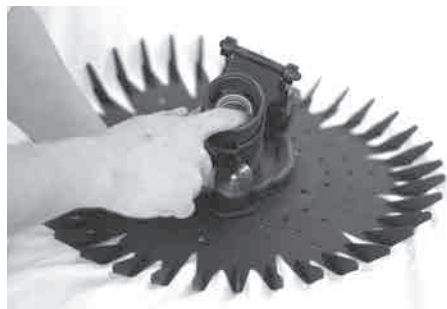
Step 9 Once diaphragm is correctly positioned push out folded end to fully open diaphragm tube.
