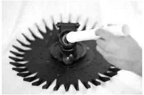
Step 2 Remove inner extension pipe from diaphragm.
