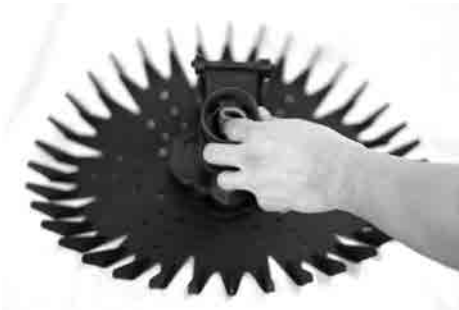
Step 3 Squeeze top edge section of diaphragm together and push down.
